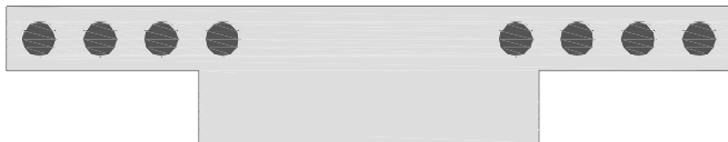
Rear T-Bar with (8) 4 in. Round Light Holes IC975004-14
