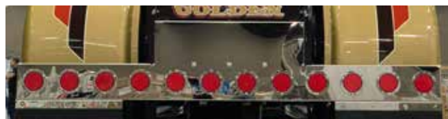
Reverse T-Bar with (6) 4 in. Round Light Holes and Recessed Airline Box with Trailer Air & (1) 7-Way
